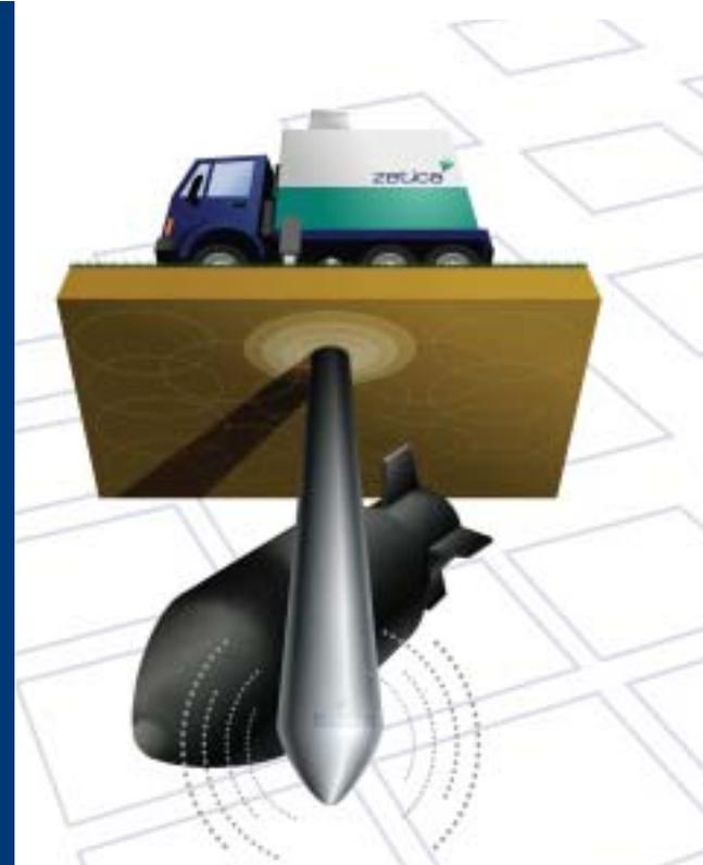
Zetica provides expert services for UXB detection and clearance. A vital part of Zetica's Sitesafe service is the MAGCONE probing system. This accurately detects large air-dropped UXB to their depth of rest, which is typically up to 15m below surface, depending on soil conditions. Contact us if you need this depth to be calculated for a specific site.
